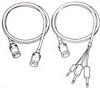
Two kinds of connector. Left: With two 'DIN' plugs. Right: With a 'DIN' plug and three 'jack' plugs.
